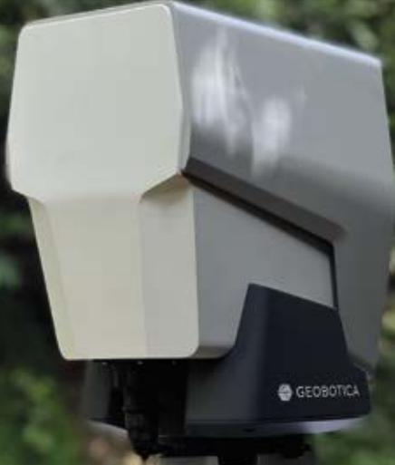
GeoLidar uses lidar combined with artificial intelligence to reveal ground movements to millimetre-scale precision.
